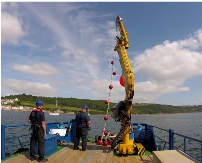
This HLF funded project includes the trialling of an eco-friendly mooring which is designed to keep the chain off the seabed. The National Marine Aquarium deployed this early in the summer in Cawsand Bay and will be monitoring its impact on the seabed over the coming year. If successful then this could offer a solution to reducing impact of moorings within the seagrass beds.
